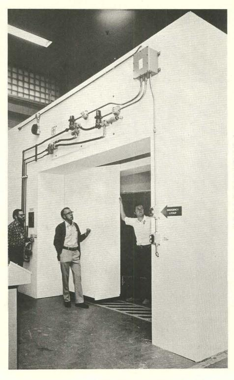
TO SAFEGUARD nuclear material at an assembly or manufacturing location, Marv Plugge, George Duke and Martin Kodlick (all 1751) have developed this hydraulically or gravity operated vault door which can be remotely or locally closed. Door has many features, including electronic coded switch for access.
